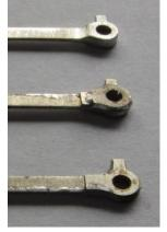
12 Open up the crankpin holes in order that the crankpin bushes will rotate in the rod. This can be done with a reamer, broach or a fine Swiss file.
